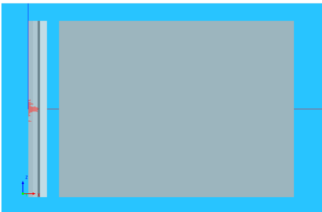
Figure 4d: Penetration (none) of 80 mm Diameter Shape Charge Through Hypothetical Armor Recipe into RHA Slab at 230 cm Standoff.
